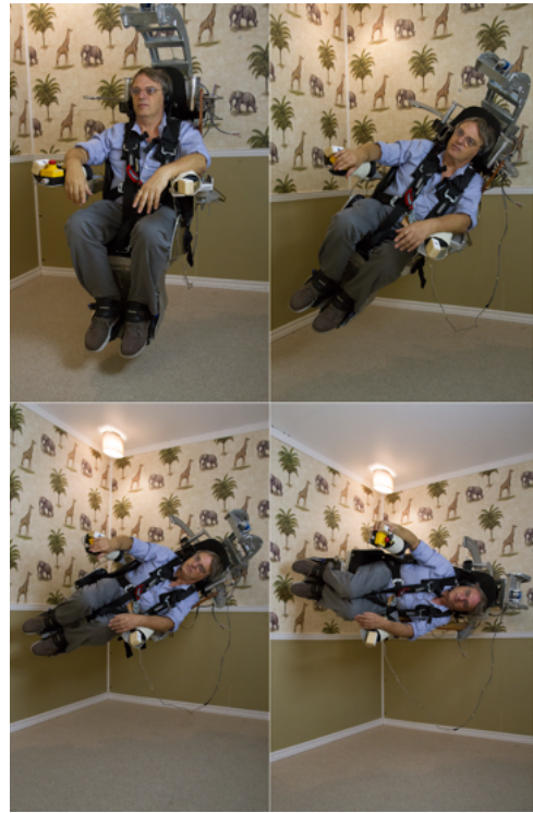
Fig. 2. The Tumbling Room enables motorized rotation of either the room or the observer (or both). In either case, under continuous rotation the observer typically perceives full 360-degree self-rotation (right). The room walls, floor and ceiling can be removed providing a continuous locomotion interface as the room turns. Imagery can be projected on the interior surface of the cylinder in this mode.
