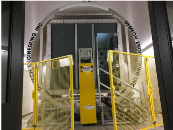
Fig. 2. The Tumbling Room enables motorized rotation of either the room or the observer (or both). In either case, under continuous rotation the observer typically perceives full 360-degree self-rotation (right). The room walls, floor and ceiling can be removed providing a continuous locomotion interface as the room turns. Imagery can be projected on the interior surface of the cylinder in this mode.
