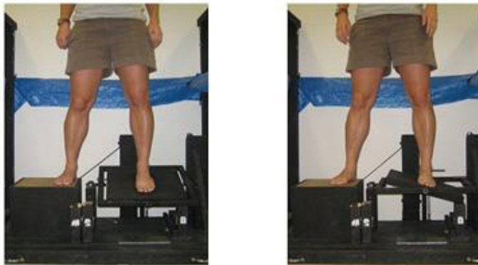
Figure 5. Active Movement Extent Discrimination Apparatus (AMEDA) for testing sensitivity to differences in extent for ankle plantarflexion and inversion movements. The physical stop blocks labeled ‘D’, ‘M’ and ‘S’ set the Deep, Mid, and Shallow distances down from horizontal, at 14, 11 and 8 degrees respectively. The aluminum plates, in a row at the front of the apparatus, provide a set of depths to discriminate for each block.
